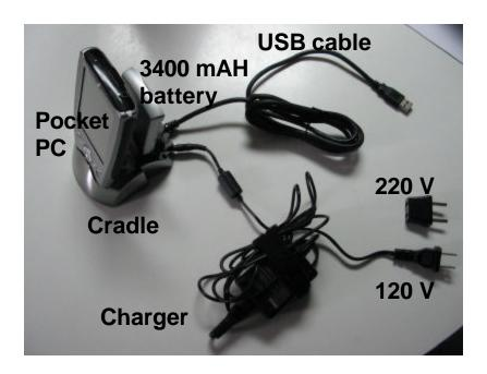
As you will see, the charger can be plugged to a 120 V or a 220 V outlet thanks to the adapter. You can also use it to download data to your own personal computer. To do so, use the USB cable.
