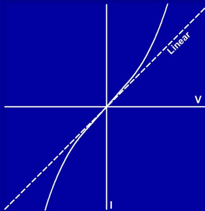
There are a number of methods of exploiting this nonlinear conduction property as a possible exploration tool.
