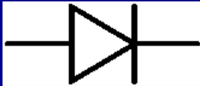
**The modern circuit symbol for a diode originated as a schematic drawing of a cat's-whisker detector**
