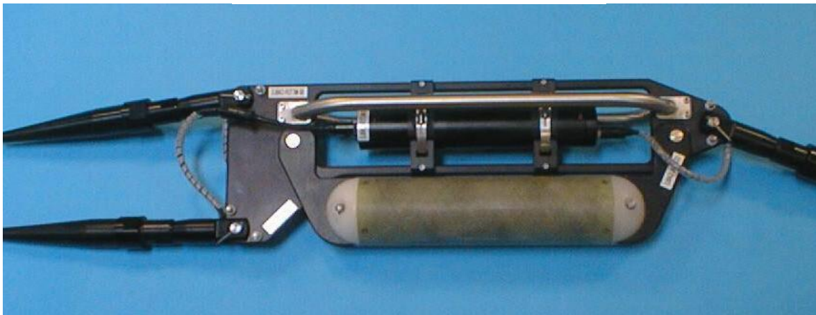
Figure 9. Telemetry tow bar with interconnect and tow cables attached.
