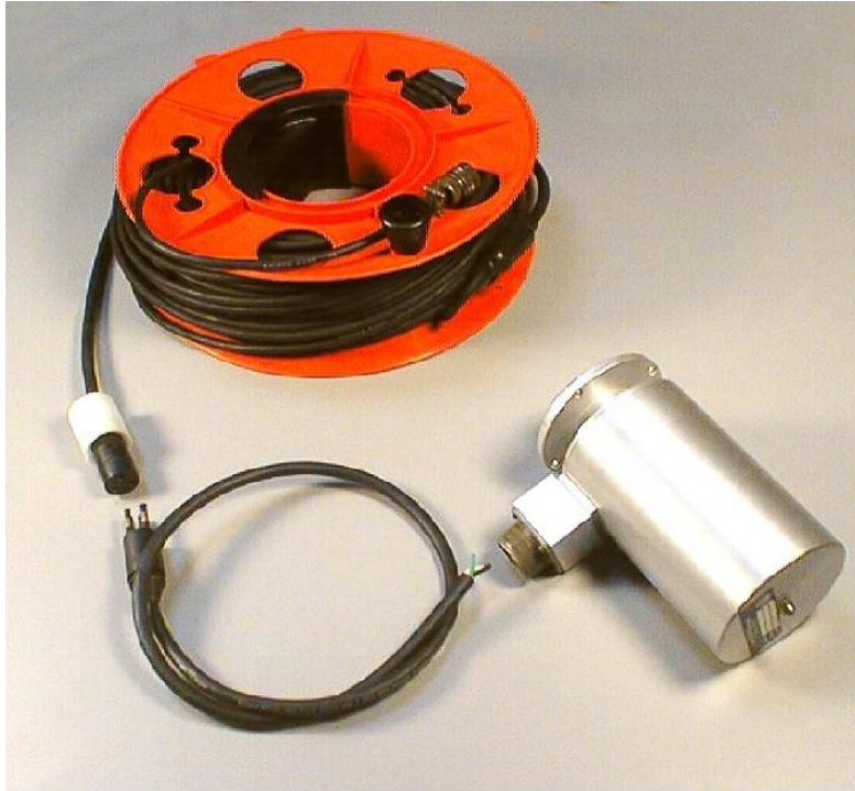
Figure 6. On-Board Cable, interconnect cable, and typical Slip ring assembly.
