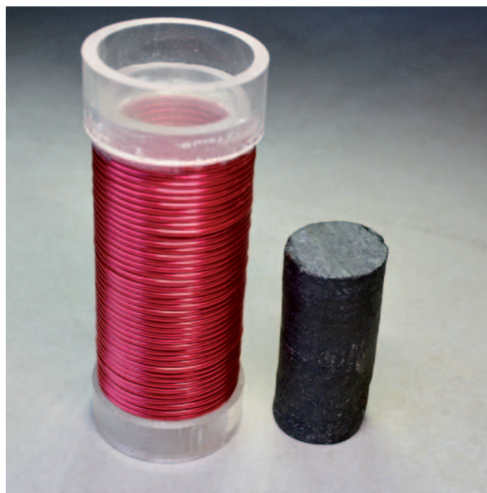
Figure 3. An induction coil of the type used in the conductivity measurements. The wire winding is 70 mm long \times 30 mm internal diameter. A conductive core inserted in the coil causes a change in its resistance, \Delta R , which is measured on an impedance bridge. If the core is magnetic it also causes a change in the coil inductance, \Delta L . From these quantities electromagnetic conductivity and magnetic susceptibility are derived (Yang and Emerson, 1997). The measurements are usually run in the kHz to MHz range (below the onset of skin effect). An air gap correction would be necessary if this method is used for a mag k measurement. The 54 mm long, 25 mm diameter Mn oxide test core shown is sample 9 with an 8 S/m EM conductivity and 114 \times 10^{-5} SI mag k . The core is porous and siliceous.
