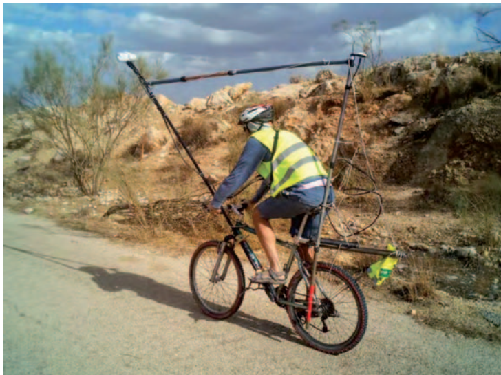
Figure 2. Uri Schattner from the University of Haifa testing the bike mounted magnetometer system. Picture courtesy of Eos/AGU.
