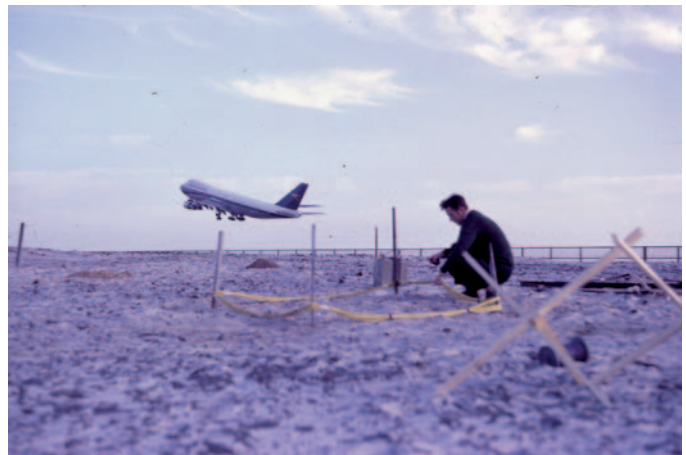
Figure 10. Ordnance detection with small multiturn loops, Port Botany.
