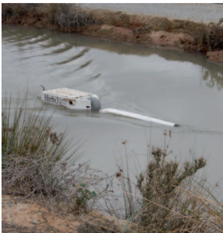
Figure 1. New receiver/transmitter electronics package being towed along an irrigation canal. The electrode array is being towed along the canal bottom and is not visible.
