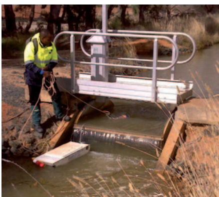
Figure 2. Electronics and array being dragged through typical canal obstacle. Small regulators, like these, and other obstacles may occur every 100 m along a typical canal.
