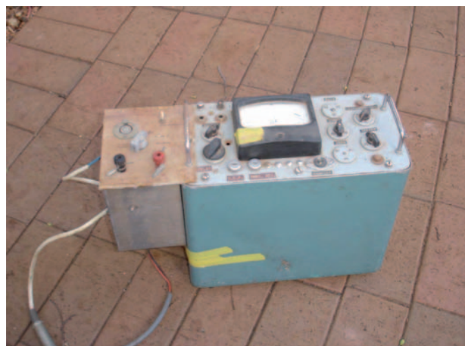
Figure 3. MPPO-1 modified by WMC with larger battery pack to provide higher transmitter currents. This instrument now resides in the ASEG Museum (courtesy John Coggon).
