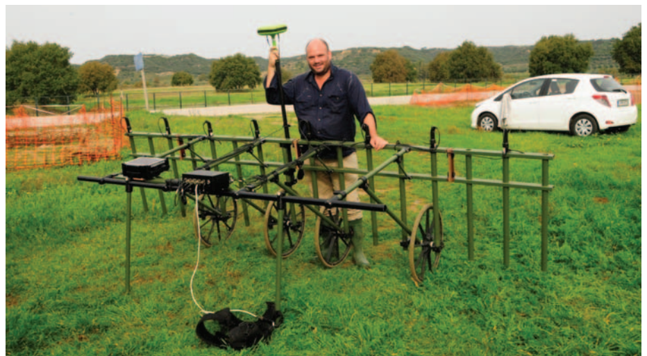
Figure 1. The author in the field with a multi-sensor gradiometer at the classical Greek site of Elis.
