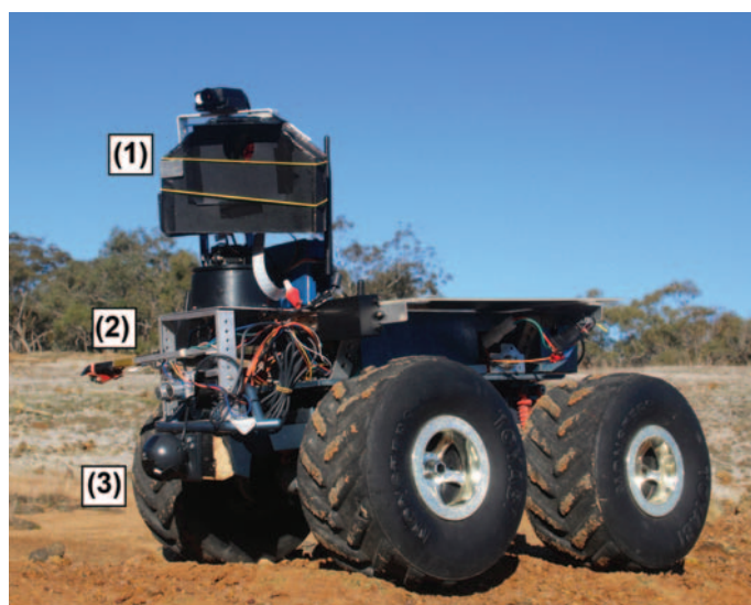
Figure 1. The Little Blue rover has been trialled in engineering tests in the Northern Flinders ranges. The rover is equipped with remote sensing and geophysical instruments for sampling the environment around it. Labelled instruments are: (1) multispectral camera; (2) non-contact IR sensor on a swing arm; and (3) macroscopic camera for close-up regolith investigation.
