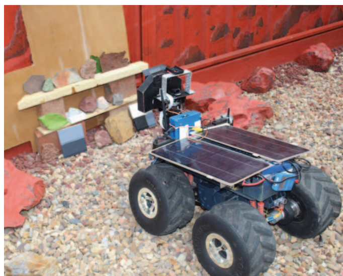
Figure 4. An important part of developing open source instruments is calibration. To this end a custom Mars yard and calibration target has been built to characterise instrument performance.
