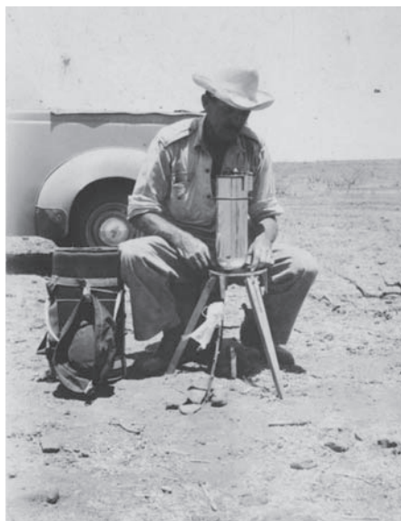
Lew using a Worden gravity meter for oil exploration in the Oaklands Basin for AOG in the late 1950s.
