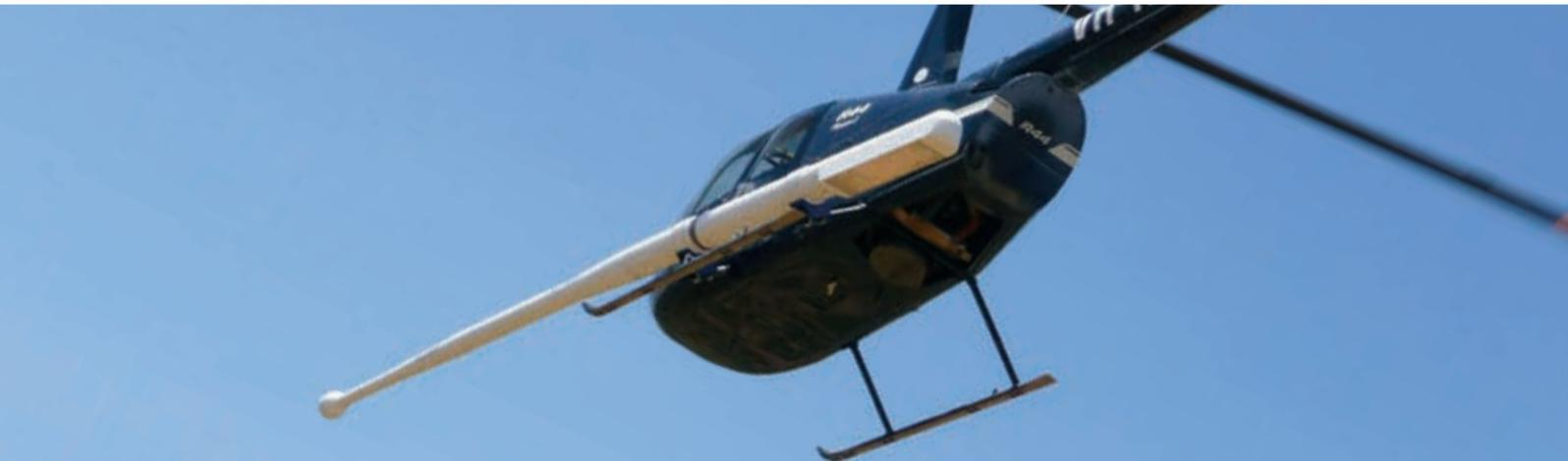
World first piston engine helicopter stinger installation for low cost, high quality airborne radiometric and magnetic data collection
