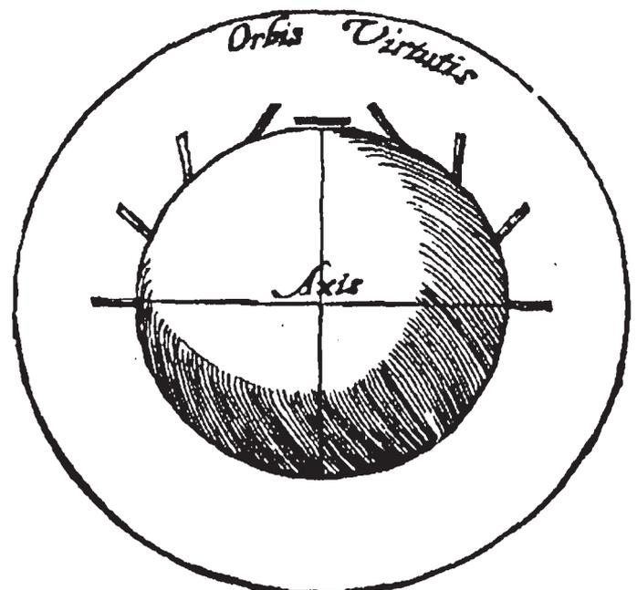
**Figure 4.** Gilbert's lodestone sphere demonstrating the earth's magnetism by the variation in inclination of fine iron needles. *Orbis virtutis*: sphere of force – limit of *terrella*'s magnetic field.
