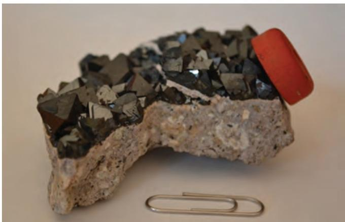
**Figure 1.** A magnet will stick to these collector-grade magnetite octahedra from Bolivia, but they will not pick up a paper clip.
