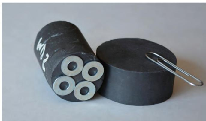
**Figure 6.** Tennant Creek Ironstone core showing the magnet effect which is patchy and not manifest on all the core surfaces.
