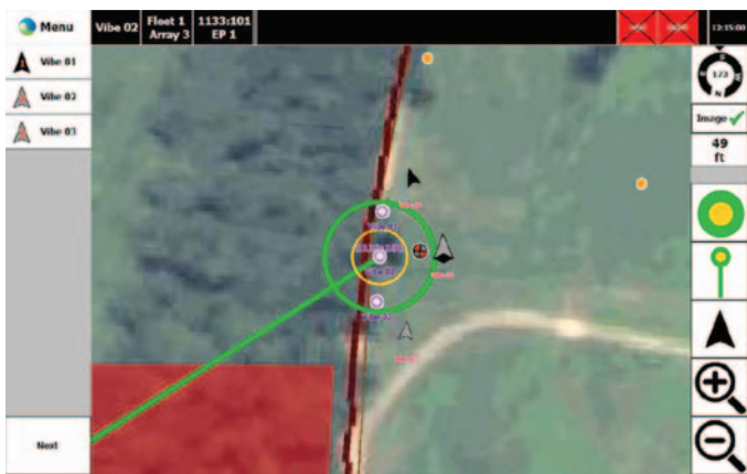
Fig. 4. Screenshot of stake-less navigation, the planned source positions are shown by the circles at the centre of the screen with the current positions of three vibrators (shown as arrowheads) to the right. (Image courtesy of INOVA.)
