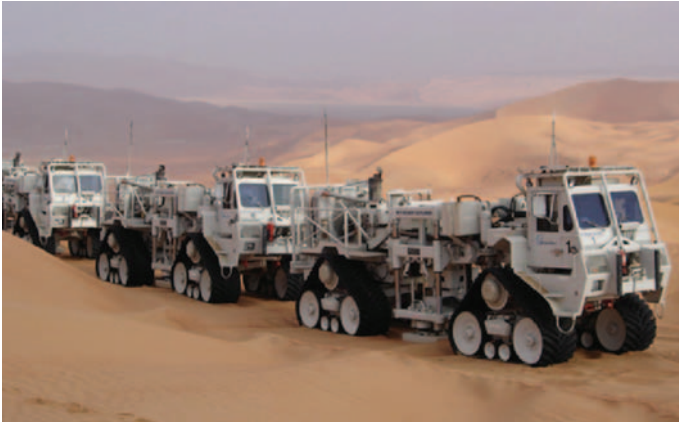
Fig. 9. Rubber tracked DX80 80 000 lb vibrators. (Image courtesy of WesternGeco.)
