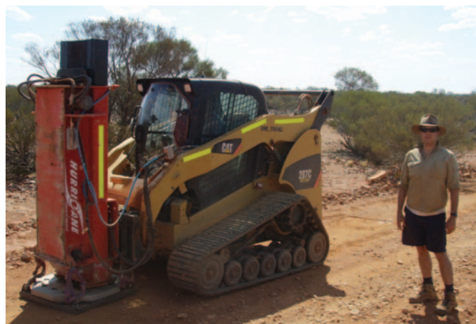
Fig. 4. Curtin University's accelerated weight drop seismic source at Abra.
