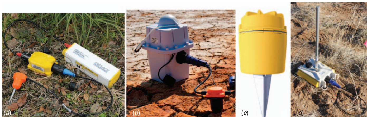
Fig. 6. Examples of cable-less recording systems. (a) OYO Geospace GSR with separate geophone, recording unit, and battery (image courtesy of OYO Geospace), (b) Sercel UNITE node with an internal battery and separate geophone string (image courtesy of Sercel), (c) ZLand with all components integrated, the unit is 15.9 cm high without the spike (image courtesy of FairfieldNodal), (d) Wireless Seismic RT 1000 unit, capable of sending data in real-time via a radio network. (Image courtesy of Wireless Seismic.)
