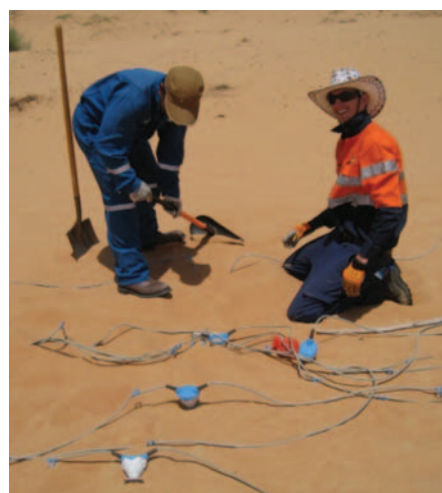
Fig. 2. Burying the UniQ geophone accelerometers.
