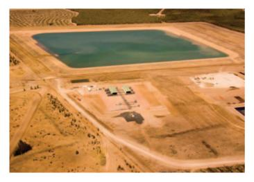
**Fig. 5.** Aerial view of Tipton West CSG Field showing dam for by-product water and compressors (Arrow Energy photo).
