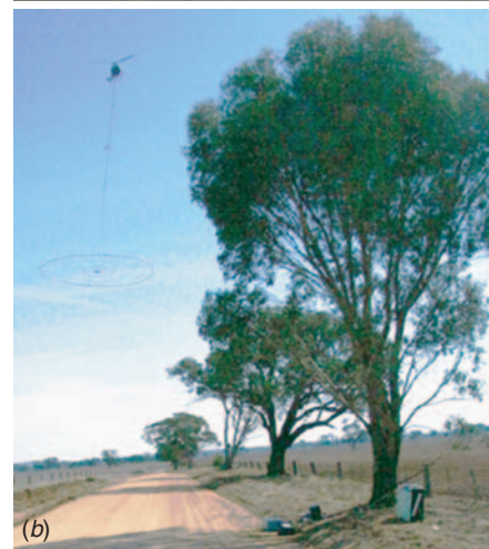
Fig. 10. (a) VTEM takes off at Stawell Airport. (b) VTEM with its towed 26 m loop flies down Sweeney's Lane at the Eastern end of Line 1 with the RMIT monitoring station set up under the tree.
