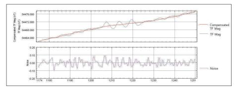
Fig. 5. GeoRanger 1.32 nT Figure Of Merit flown at MOA Boardman Oregon in August 2004.
