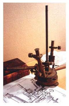
Fig. 4. A surviving Reisetheodolit. Lamont manufactured forty five of these instruments. Image courtesy of Professor Heinrich Soffel, University of Munich.
