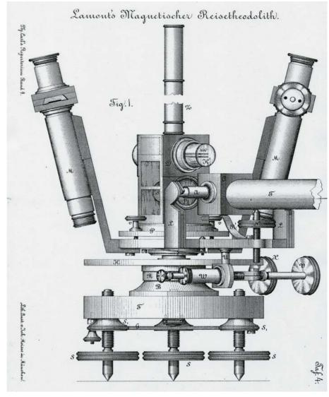
Fig. 5. Lamont's combined declination, inclination and horizontal intensity "Reisetheodolit". Neumayer measured all of his Victorian field measurements using a similar instrument. Image courtesy of Professor Heinrich Soffel, University of Munich.
