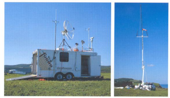
Figs. 3 and 4. GeoRanger small footprint ground systems can be set up inside an acre or on the deck of a marine vessel (control unit on left and retrieval system on right).
