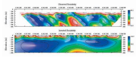
Fig. 9. Line 738100E, resistivity model (after Anderson, 2004).
