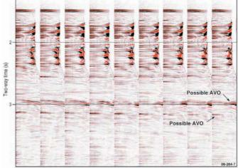
Fig. 7. 4th Order NMO + eta corrected Common Mid-Point gathers around the possible AVO anomalies.
