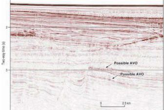
Fig. 5. Mid angle stacked section of the possible AVO anomalies.
