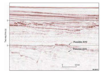
Fig. 6. Far angle stacked section of the possible AVO anomalies .
