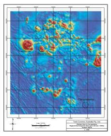
Fig. 6. Image of the Analytic Signal, showing the responses associated with Olympic Dam, Acropolis, Wirrda Well and Carrapateena.
