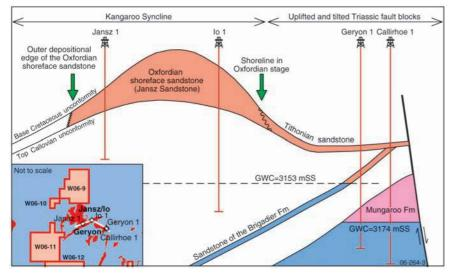
Fig. 3. Schematic cross section, showing two separate gas pools in the Jansz 1, Geryon 1 and Callirhoe wells (Korn et al., 2003; Jenkins et al., 2003).
