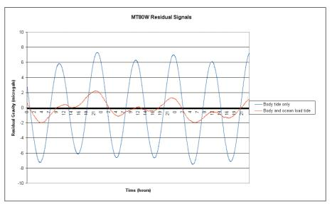
Fig. 4: This diagram shows the residual tidal signal after the predicted Earth tides, obtained from the program MT80W, have been removed from the superconducting gravimeter data. The blue line shows the residual signal if only the body tide is predicted, while the red line results from the removal of both the body and ocean load tide predictions.
