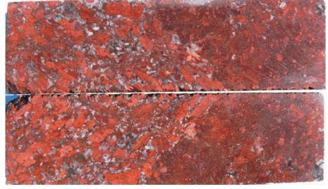
Fig. 3. Haematite altered granite breccia with fine grey haematite clasts disseminated throughout an earthy haematite matrix.
