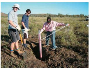
Fig. 2. Monash postgraduates assisting Seong Kon Lee with site preparation and recovery of an MT sensor coil.
