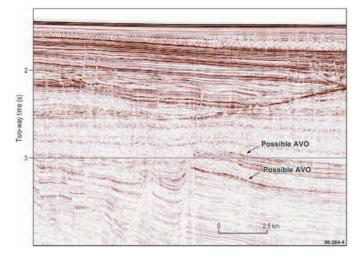
Fig. 4. Near angle stacked section of possible AVO anomalies.
