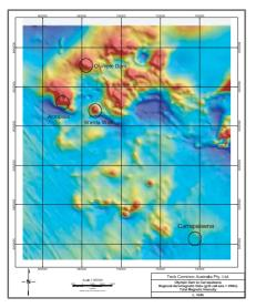
Fig. 5. Image of Total Magnetic Intensity, showing anomalous responses associated with Olympic Dam (1600 nT), Acropolis (5500 nT), Wirrda Well (1800 nT) and Carrapateena (200 nT).
