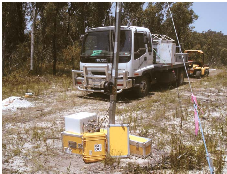
Fig. 1. ANSIR MiniVib (IVIT 15000, 6,000 lb configured in P-wave configuration) and recording system operating during the BHP Billiton Illawarra Coal project near Appin, NSW.
