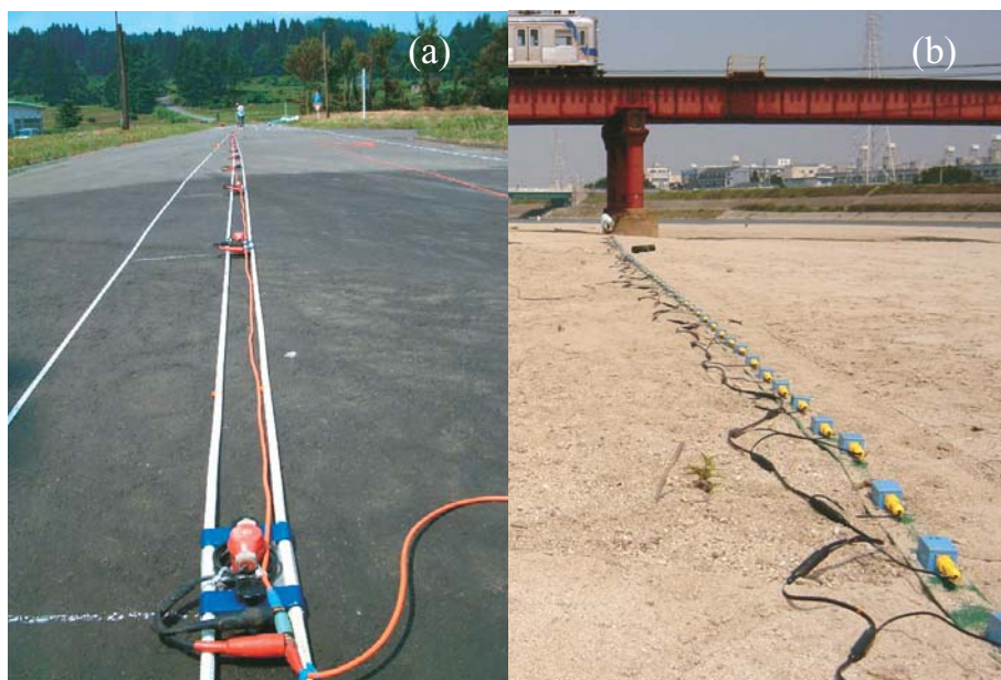
Fig. 4. (a) 24-channel landstreamer on asphalt, with standard 4.5 Hz vertical component geophones, and (b) 96-channel landstreamer on sand, with custom made transverse component geophones.
