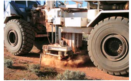
Fig. 2. Close up of a vibrator, note the geophones planted nearby.
