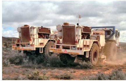
Fig. 1. Two of the Hemi 60 vibrators, raising the dust near Broken Hill.
