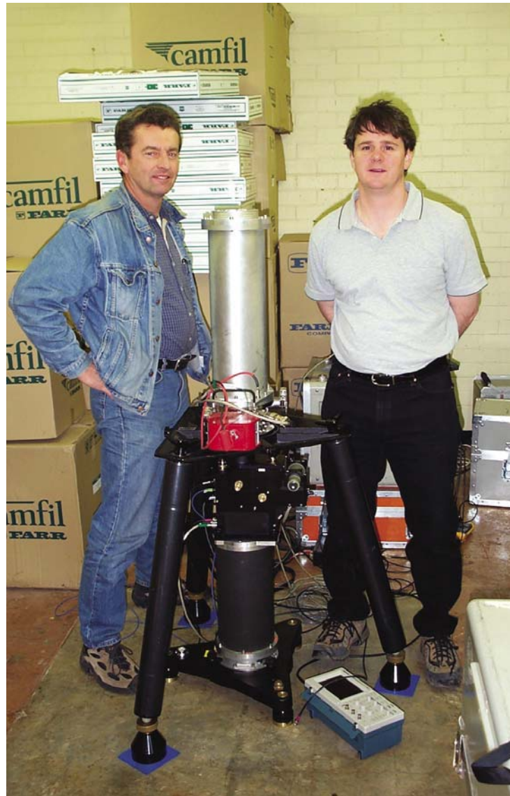
Fig. 4. FG5 gravimeter setup in shed at Dampier WA during June 2003 FG5 absolute gravity survey. John Peacock from Fugro Ground Geophysics is on the left. He assisted Kip Buxton from Micro-g Solutions on the right, during June 2003 FG5 absolute gravity survey.
