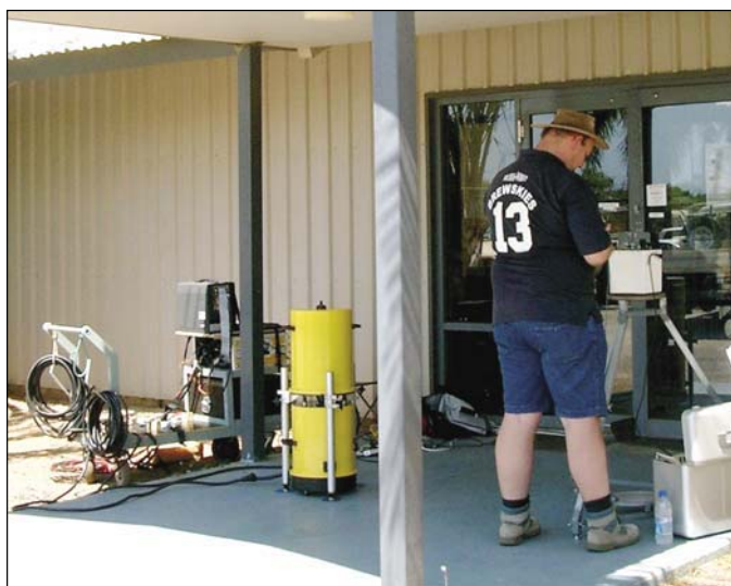
Fig. 2. The A10 portable absolute gravimeter set up at a Fundamental Gravity Base Station. The yellow device is the sensor and the trolley behind houses batteries, electronics, and computer interface for the instrument. It also serves to transport the complete system when it is not set up in a vehicle. The vertical gravity gradient is being measured alongside the A10 using a LaCoste & Romberg gravimeter.
