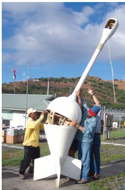
Fig. 8. Assembling NewTEM Rx bird in 2004 in Indonesia.
