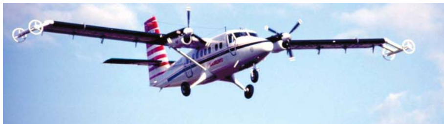
The deHavilland Twin Otter aircraft being used by the British and Finnish Geological Surveys. The wheel-like devices are the transmitter and receiver coils for the EM system. The magnetic sensors are housed inside the wingtip mountings.
