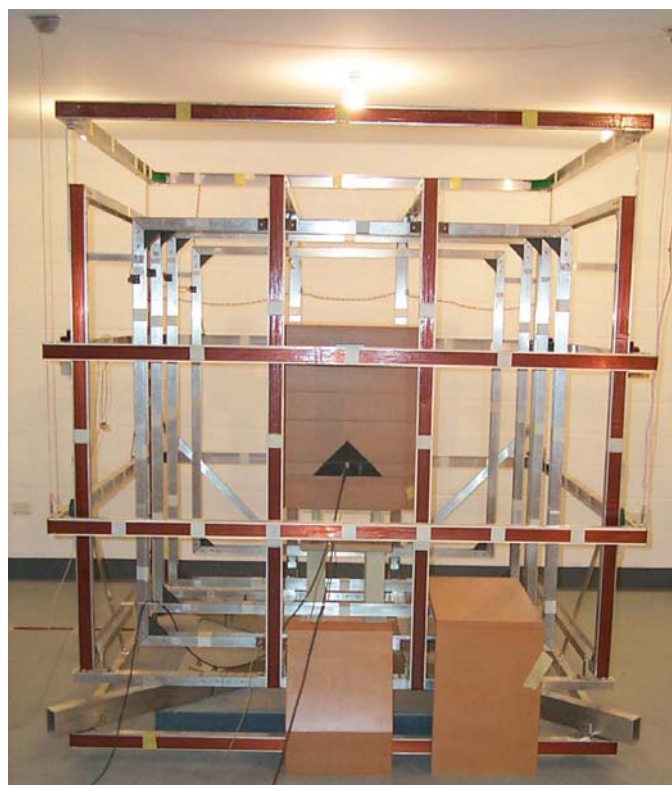
Magnetometer in insulated compartment being tested within the large three-axis magnetic calibration coil system at the Canberra Magnetic Observatory
