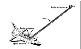
Fig. 1. The SRTM dual radar antenna setup on the Shuttle spacecraft.
