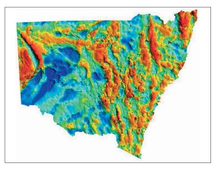
Fig. 2. Bouguer gravity data of New South Wales after isostatic correction is applied.
