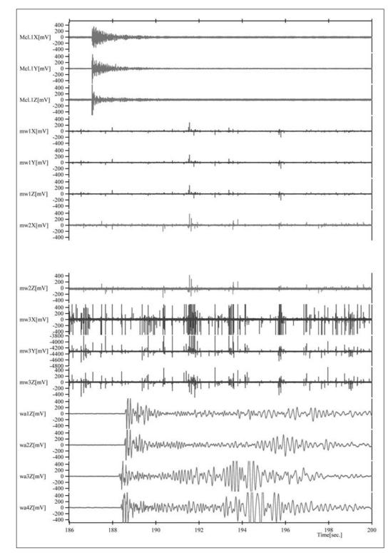
Fig. 5. Seismograms of seismic event originating from close to Habanero-1.
