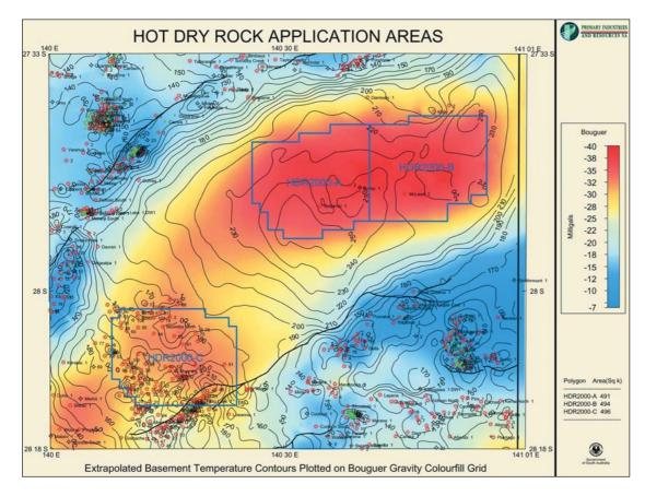
Fig. 3. Locations of HDR Exploration Leases and estimated basement temperatures plotted on to Bouguer Gravity contours.
