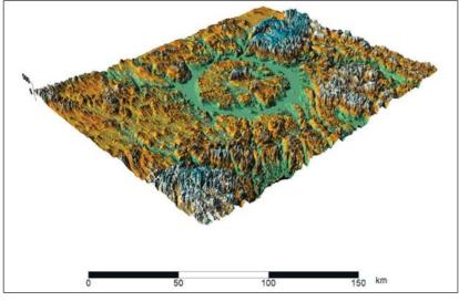
Fig. 4. SRTM DEM for the Manicouagan impact structure, Quebec, Canada. Cell size is 3 arc seconds, about 90 m, and the viewing direction is looking northeast.
