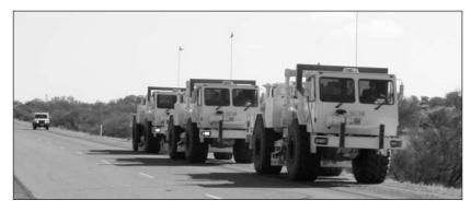
Fig. 2. The source Vibroseis trucks operating on the Woomera to Roxby Downs road.
