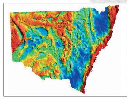
Fig. 1. Bouguer gravity image of New South Wales. Gravity data generated from Australian National Gravity Database 2003 published by Geoscience Australia.
