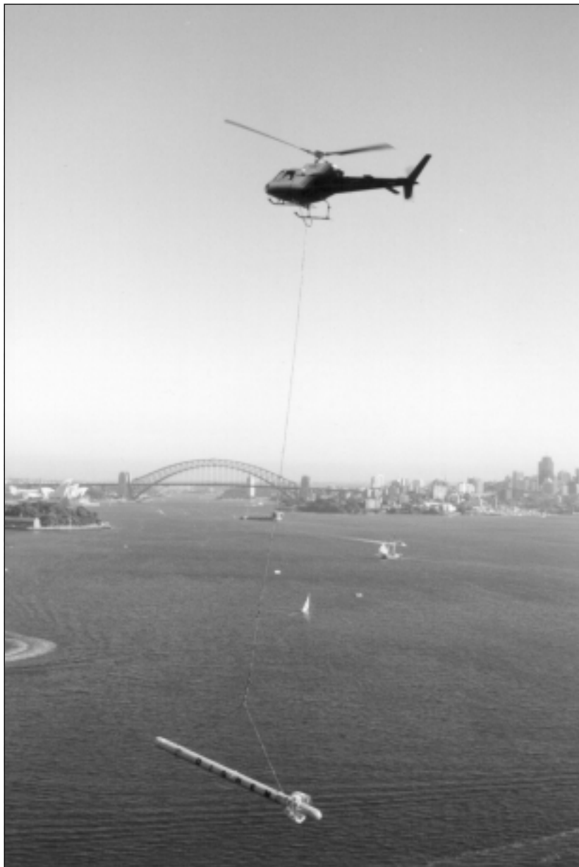
Sydney - DIGHEM helicopter, Sydney Harbour - bathymetry (Fugro Airborne Surveys).
