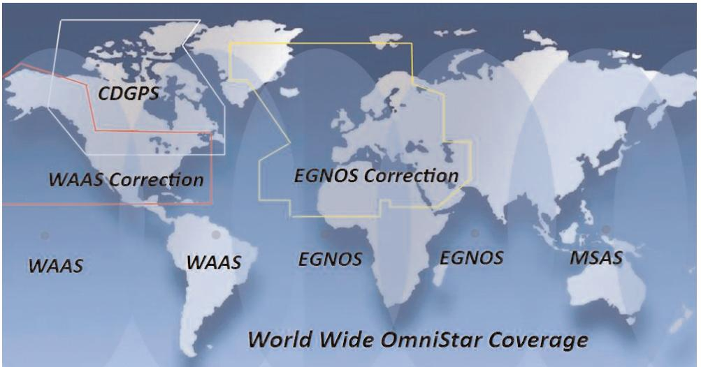
Coverage areas supported in GEM's advanced magnetometers. OmniSTAR is a global service; SBAS comprises WAAS, EGNOS and MSAS satellite systems; and CDGPS is the new Canadian standard.
