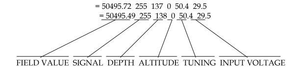
The values shown are for example only and will vary with system configuration. The first reading is the magnetometer field and its value will vary greatly if the sensor is
