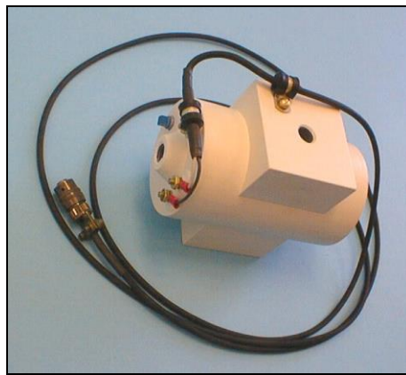
Figure 12. Bottom sensor with gradiometer cable attached
