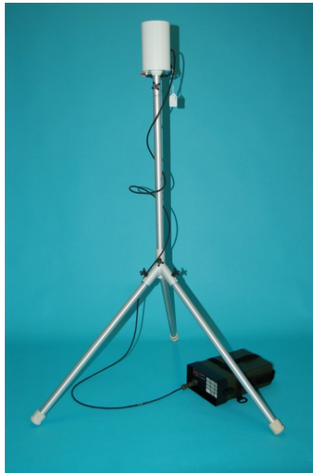
Figure 16. Base-station setup using tripod kit and G-856AX staff section
