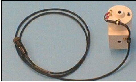
Figure 11. Top sensor with gradiometer cable attached
