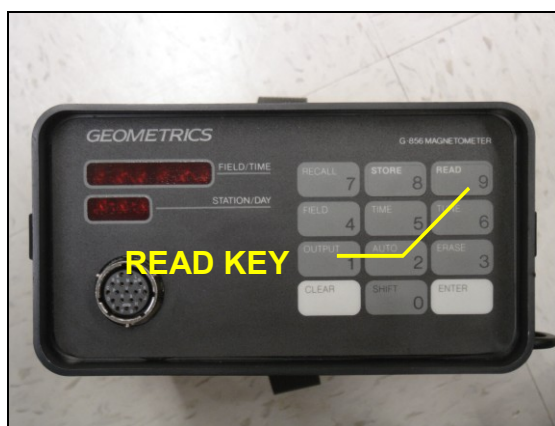
Figure 8. Location of 'Read' key on magnetometer console
