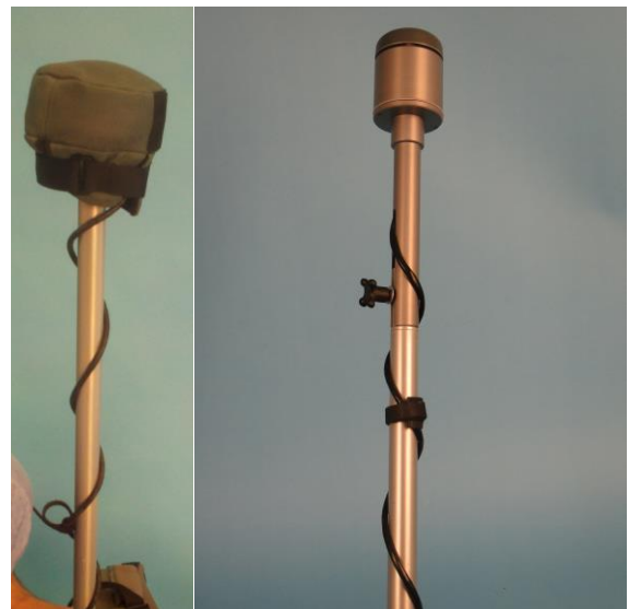
Figure 7 showing GPS cable routing Left: NovAtel GPS Right: Tallysman GPS
