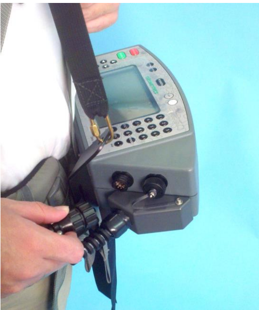
Figure 23A Insert Power Connector
