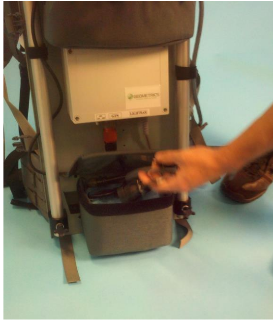
Figure 9B Locating power cable connector, mount connector on junction box power plug
