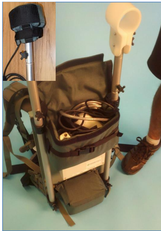
Figure 6 showing sensor and GPS antenna with NovAtel GPS Staff assembly shown in inset
