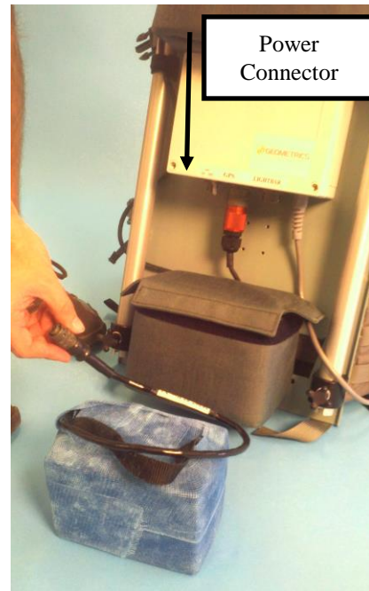
Figure 17 Locate Battery Connector
