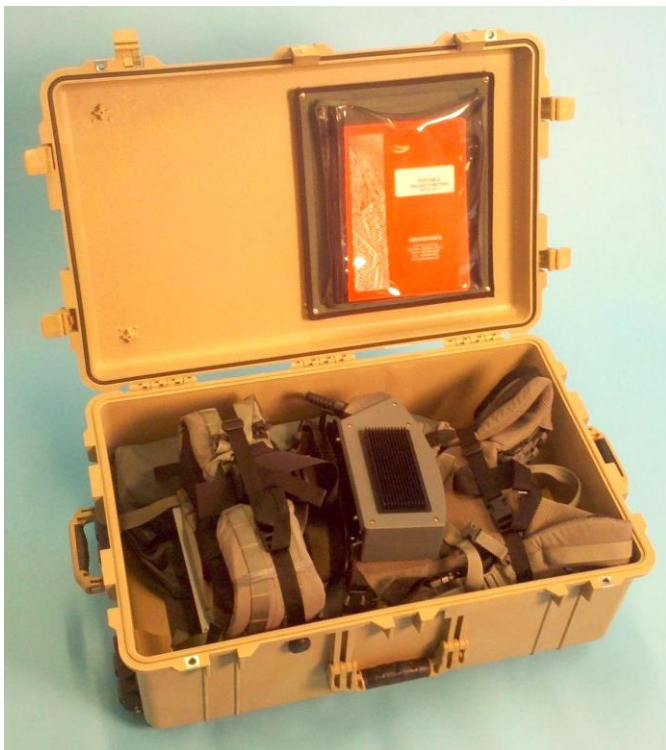
Figure 1 Shipping case with G-859AP pack frame strapped into the case. Console secured to the frame
