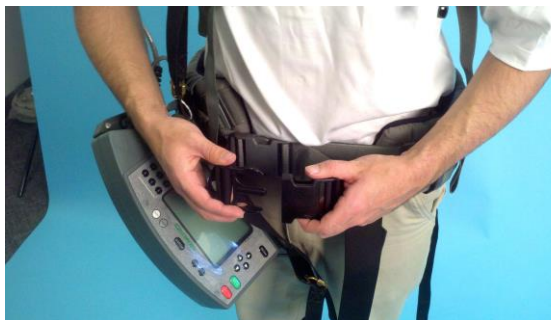
Figure 20B Secure secondary console belt
