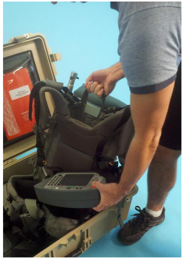
Figure 4 Remove Frame and Console from the case
