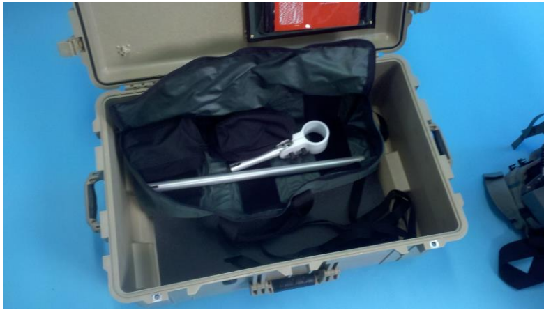
Figure 5 Sensor staff with clamp and GPS mast
