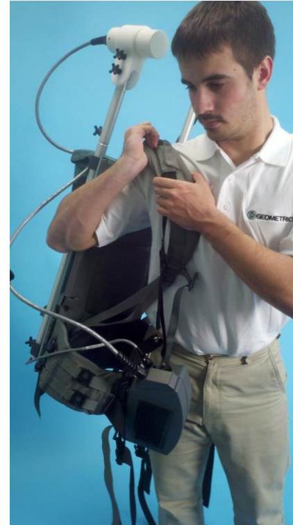
Figure 19B Swinging the pack onto the shoulder
