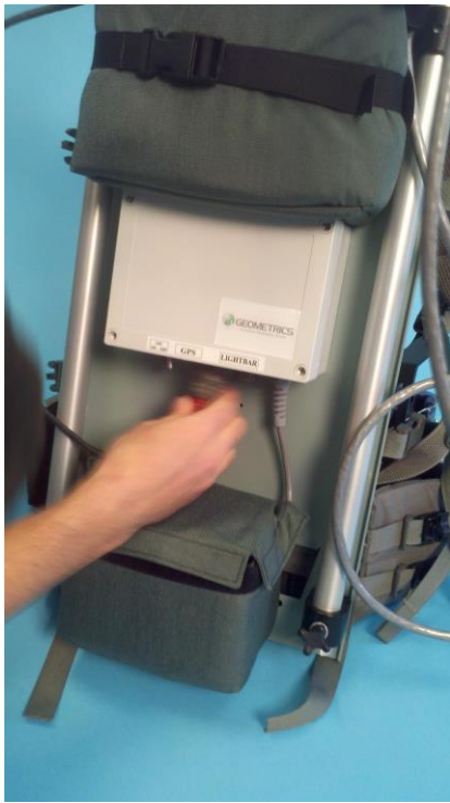
Figure 9A Attach GPS Cable to Junction box
