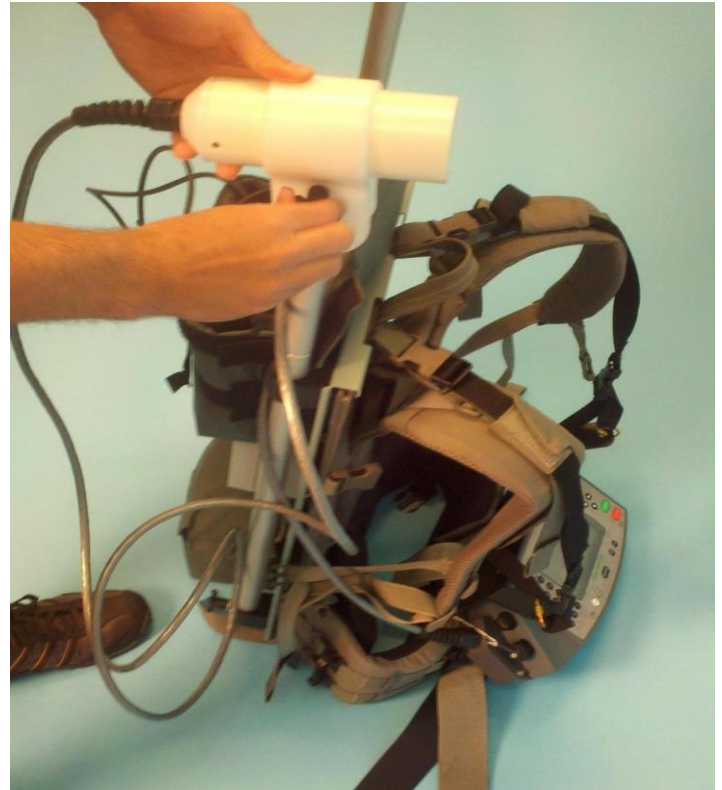
Figure 8B Tightening Sensor Clamp for Horizontal operation
