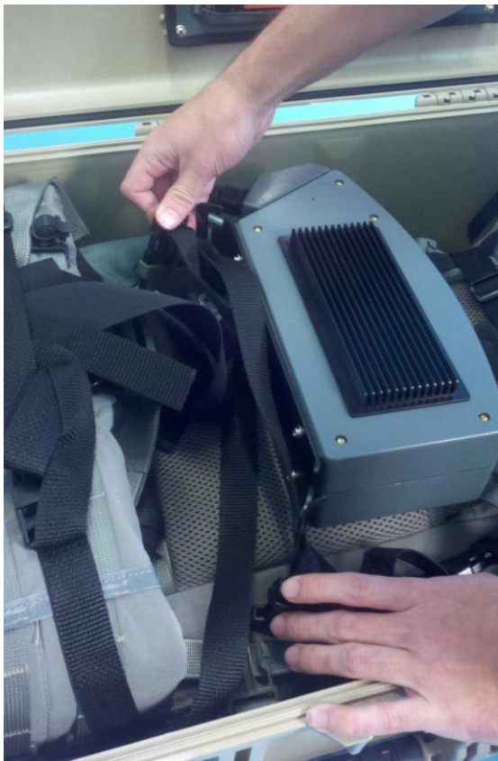
Figure 3 Remove Console security strap
