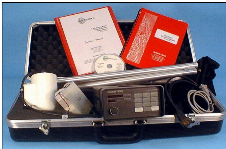
Figure 1. G-857 proton-precession magnetometer.
