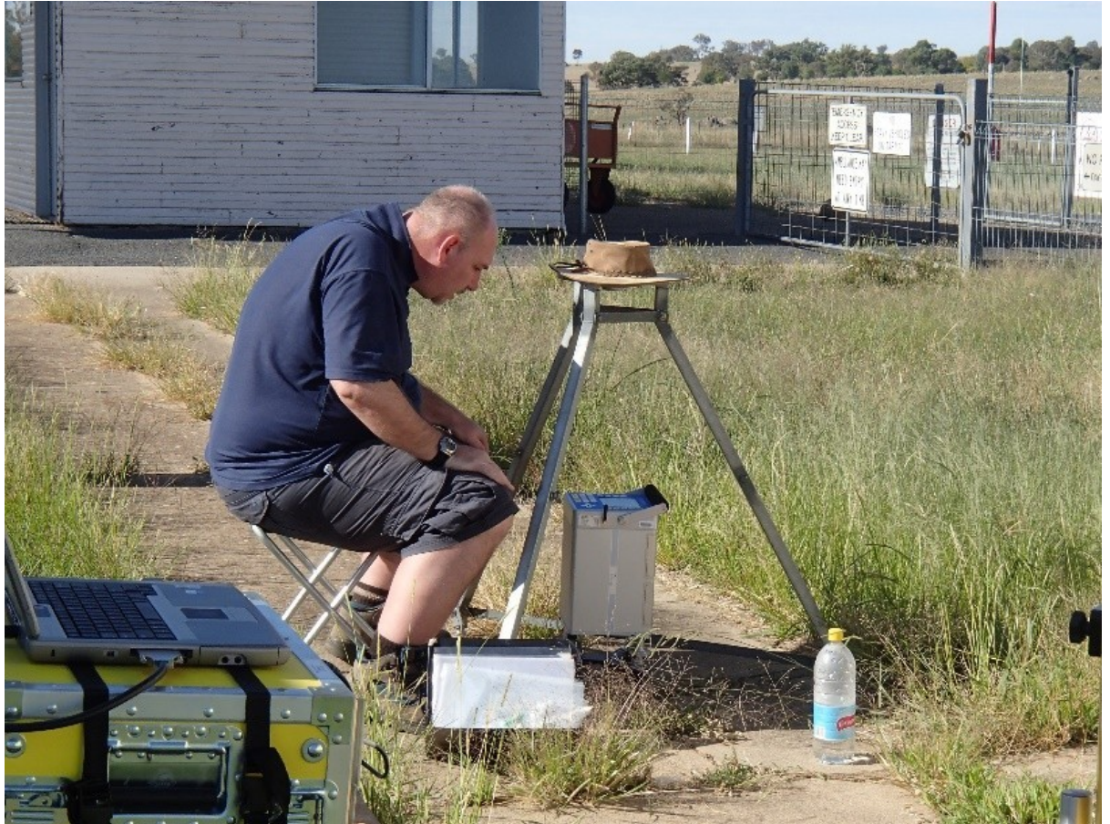
Photo: Phill Wynne using CG5 a gravity reading at an AFGN site near Young, NSW.
