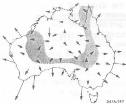
Fig. 20. Magnetic induction vectors corresponding to a period of 42.7 minutes computed at AWAGS stations from a magnetic storm on 29 December 1989. Areas where the induction vectors show large variability in size and direction are characterized by heterogeneous induction properties, and are therefore liable to large base-station errors.
