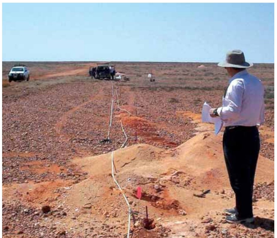
Figure 2 Jingping Zhe conducting a resistivity survey at Site 1. (Photo 404951)
