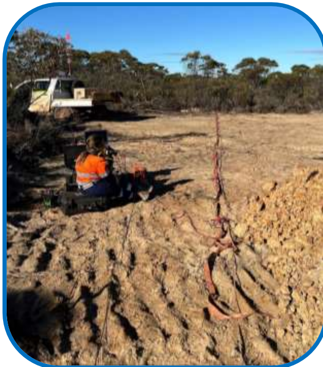
Acquiring Refraction Seismic and MASW at Mt. Holland WA
