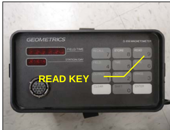
Figure 8. Location of 'Read' key on magnetometer console.
