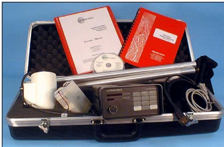
Figure 1. G-856 proton-precession magnetometer.
