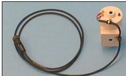
Figure 11. Top sensor with gradiometer cable attached.
