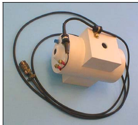
Figure 12. Bottom sensor with gradiometer cable attached.
