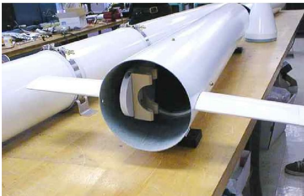
Figure A2. Airborne Stinger showing sensor mount.
