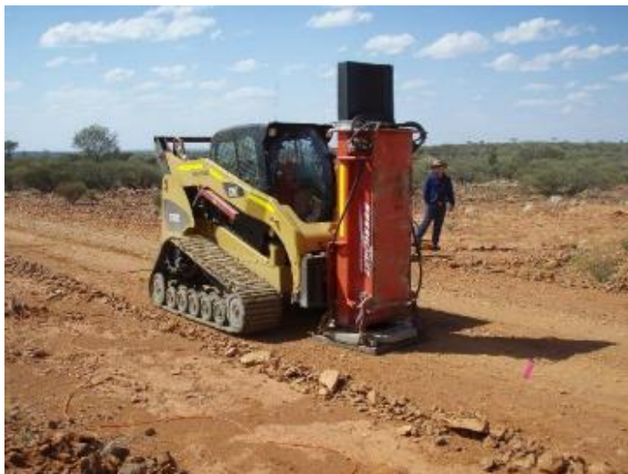
Curtin accelerated weight drop source mounted on a bobcat
