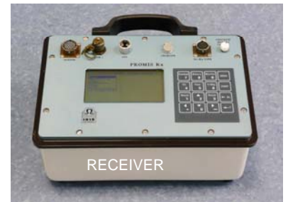
PROMIS FREQUENCY EM SOUNDING with 50m, 100m, 200m Tr-Re spacings, Orléans Loire River site, France
