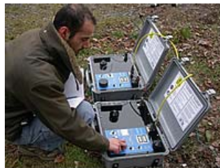
Two GDD 3600W-2400V IP transmitters linked together to increase power up to 7200W and voltage up to 4800V.
