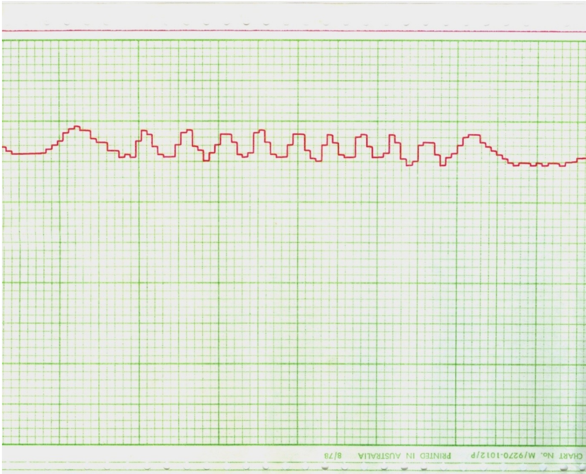
A piece of analog magnetic diurnal record from Mt Isa 1979 ex Dave Lyus 2 second sampling 100 nT fullscale which mapped a moving rotary clothes hoist beautifully.
