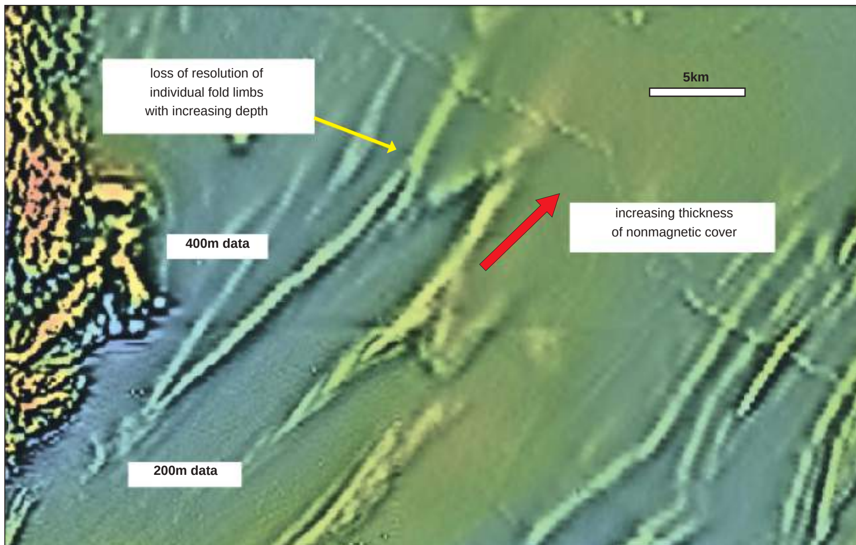
Figure 4.8: Aeromagnetic image from the Cloncurry region of the Mt Isa Inlier (Qld) illustrating the decrease in spatial and structural resolution (red arrow) with increasing depth (in direction of red arrow). Cover over the folded Proterozoic metasedimentary sequence thickens to the NE. Note also the change in resolution due to change in survey line spacing. The more detailed data in the SW corner has 200 m line spacing compared to 400 m spacing over the rest of the area. Data courtesy of Geoscience Australia and Geological Survey of Queensland.
