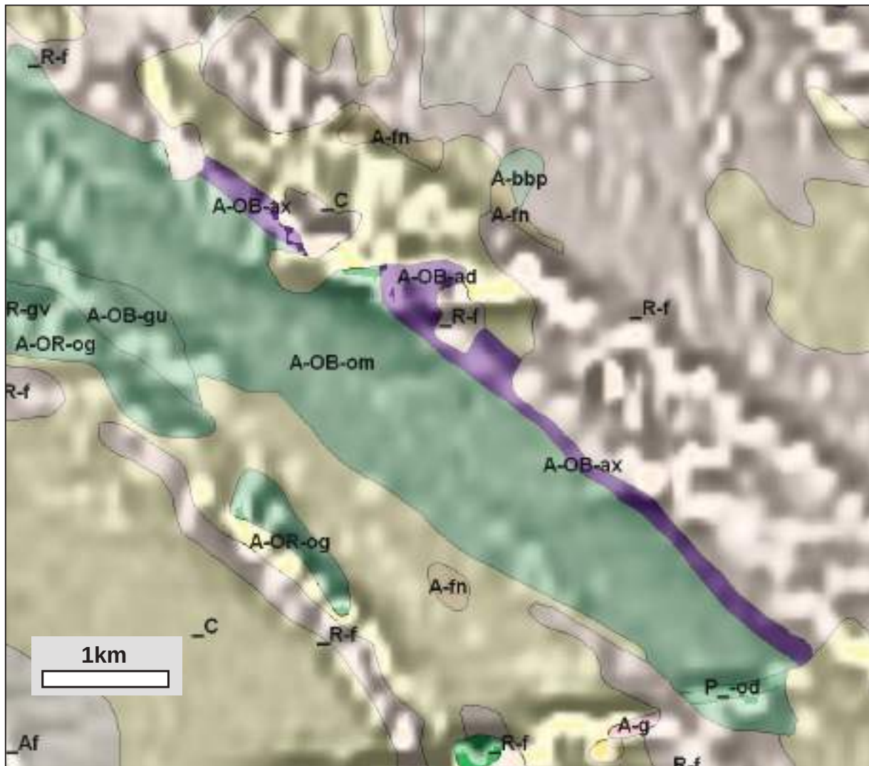
Figure 3.12: RTP 1st VD image superimposed on outcrop geology over the Archaean Ora Banda Sill (A-OB), WA. The sill faces SW and the upper differentiates, gu (quartz-gabbro/granophyre) and om (gabbro-norite) are very weakly or non-magnetic. Only the basal differentiates, ax (bronzite/norite) and ad (dunite) are magnetic. Data from GSWA open file digital databases.
