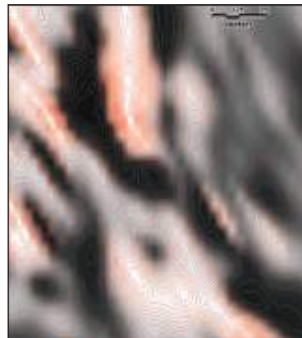
200m line spacing. Image pixel size is 10m, resampled and reinterpolated from 40 native cell size. The line spacing is 4 x the flying height and line perpendicular gridding artifacts begin to appear. The bias is now dominant in the RTP 1 st VD image. The RTP is 'useable', but the RTP 1 st VD, although 'presentable', is misleading.
