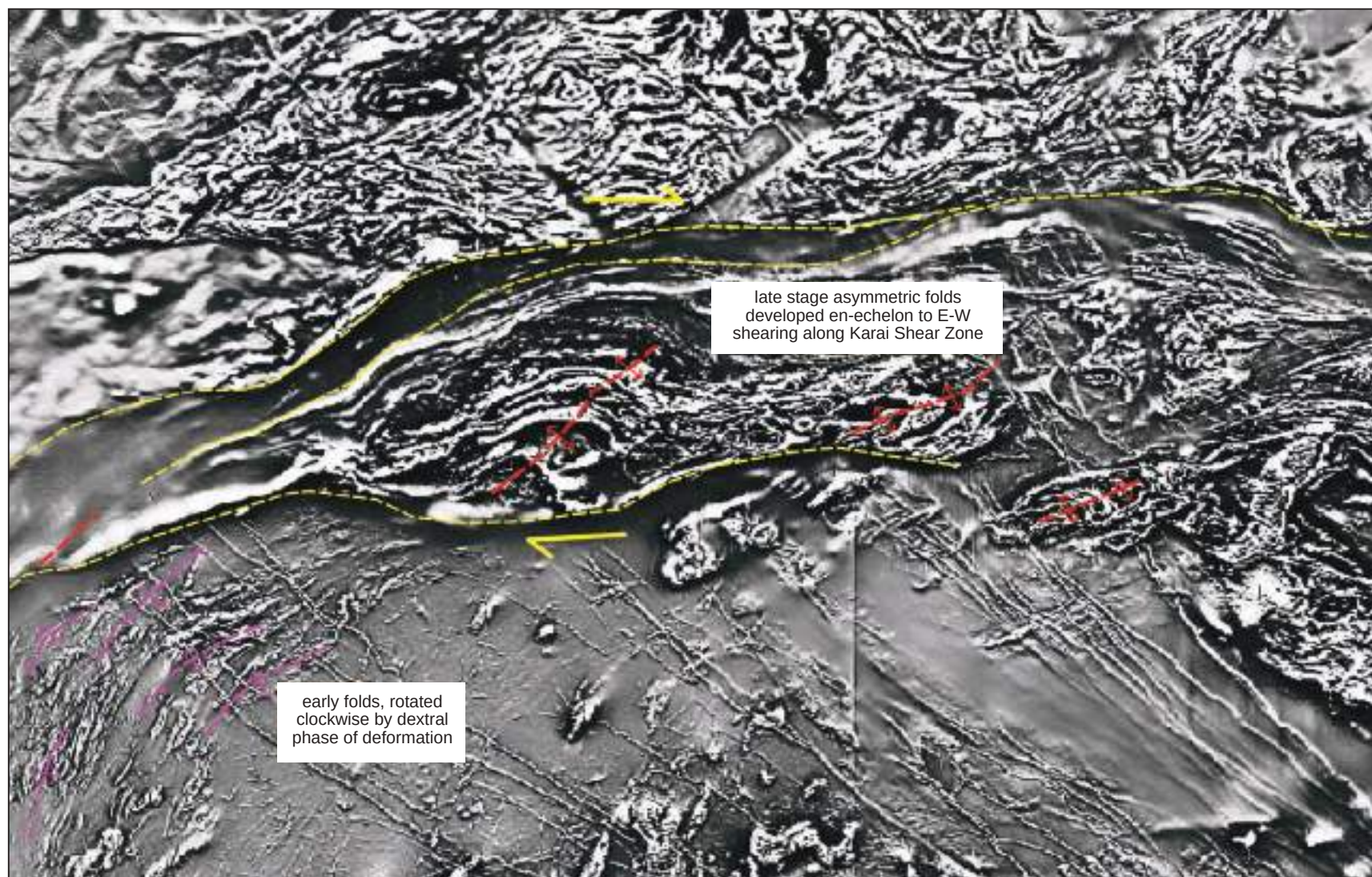
Figure 4.24: Aeromagnetic image over the Coober Pedy Ridge are of the NW Gawler Craton, SA. The traces of the Karari Fault Zone (plus associated structures) are shown (yellow dashed lines). An episode of dextral shear along this sector of the fault zone is interpreted from: a) significant clockwise rotation of early folds into the shear zone (SW corner of image – pink dashed lines); b) development of late-stage en-echelon, NE-trending asymmetric folds (central sector of image – red dashed lines). Data courtesy DMITRE.
