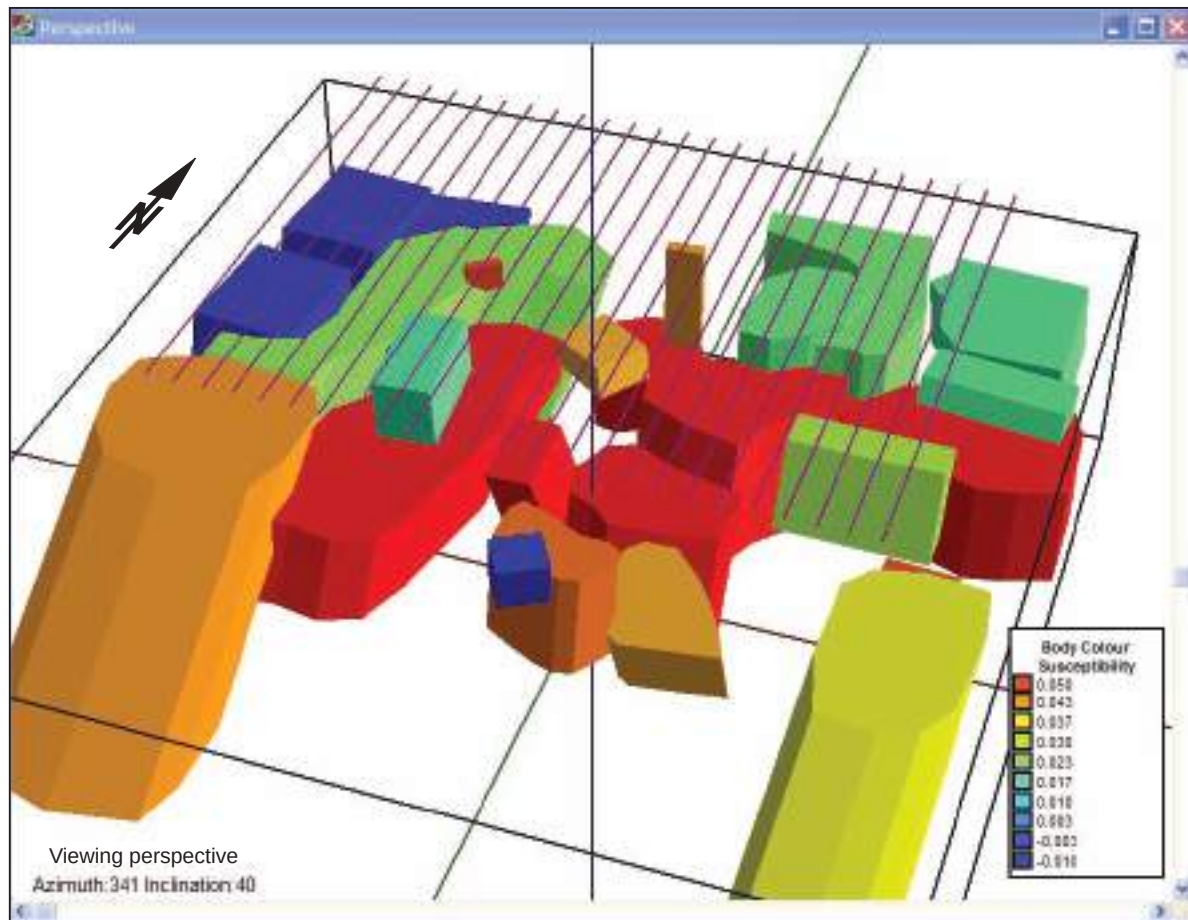
Figure 13.28: Detailed study subarea. Location of initial modelling lines and first-pass 3-D model bodies. Modelling by Z. Shi.
