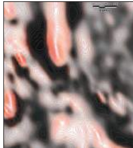
100m line spacing. Image pixel size is 10m, resampled and reinterpolated from 20 native cell size. The line spacing is 2 x the flying height but gridding artifacts are not apparent. Note the 'disappearance' of the NNE trending dyke, seen in the 50m data. This is an important 'pit-scale' geological structure.
