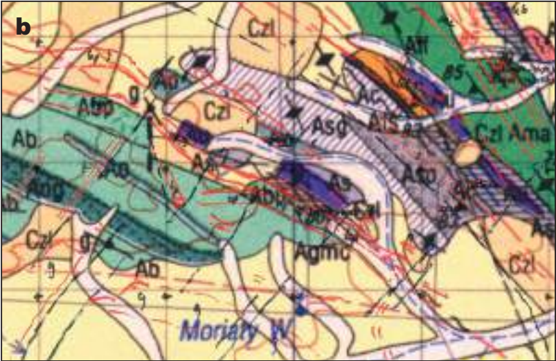
Detailed aeromagnetic observations, superimposed on outcrop geology, Grid is 1km
