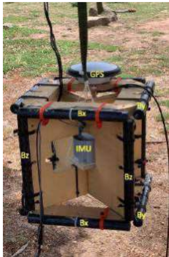
Figure 3: Test jig with 3 (x,y,z) component B field sensors with rotation measuring hardware.
