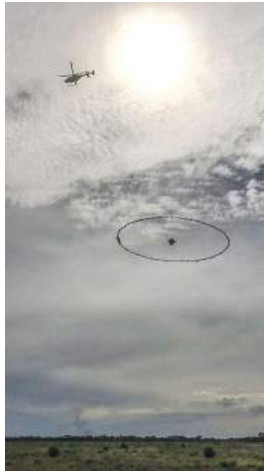
Figure 12: The transmitter in flight, with a 3 component BIPTM sensor in the centre
