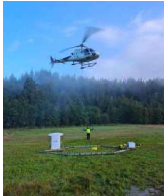
Figure 1: Picture of a miniature airborne TEM system called SkyTEM21HR used in this geotechnical ground investigation study.
