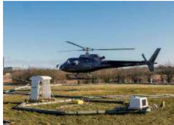
Figure 3. Scaled-down frame used for testing the drone TEM transmitter and receiver electronics.
