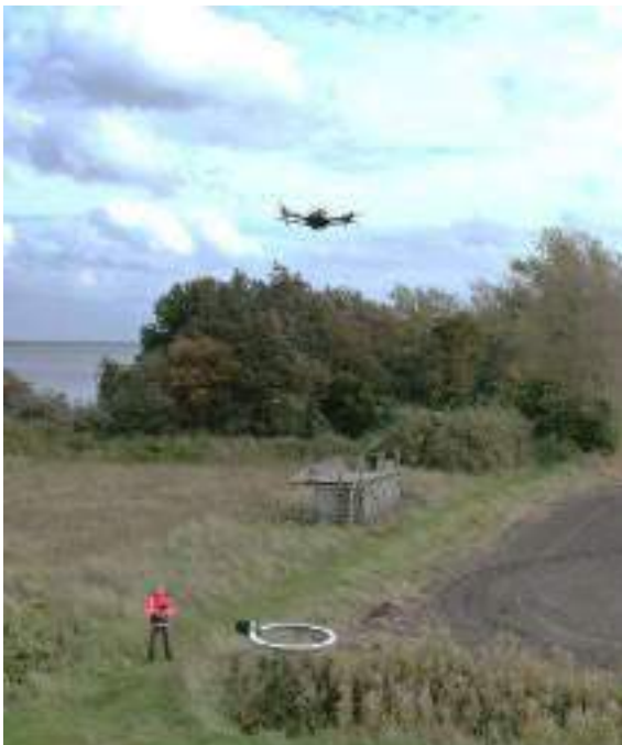
Figure 1. The picture shows a prototype of the drone and receiver coil flying at the Aalborg University drone test facility.
