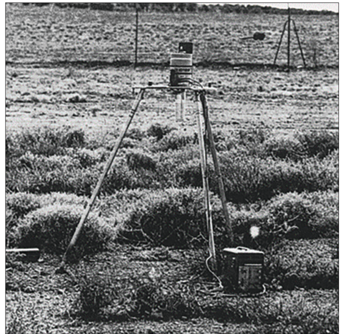
Figure 5. High purity germanium detector at Taranaki (Tipton et al. 1988).
