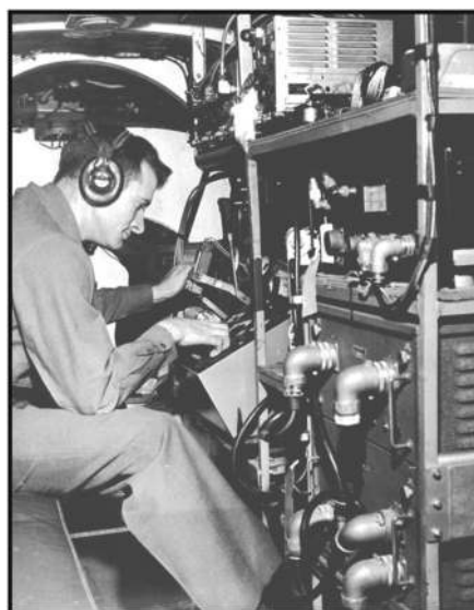
Figure 3 (Figure 86b). James Robinson Balsley of the USGS operating the magnetometer in the US Navy SNB-1 BuNo 51044, 1944-45. US Geological Survey.
