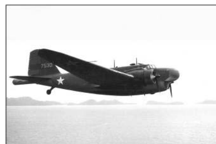
Figure 2 (Figure 48). The USAAF Sea-Search Attack and Development Unit (SADU) Douglas B-188 Bolo BuNo 07530. One of a series of photographs taken "near British West Indies and Martinique 12 July 1942". These are the earliest identified photographs of an operational aircraft with a magnetometer or MAD mounted in a "stinger". USAF. Public Domain. Various sources including NARA.
