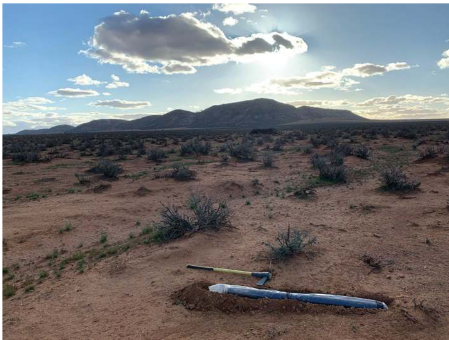
Figure 1. An induction coil to measure the magnetic field, with Anabama Hill in the background.
