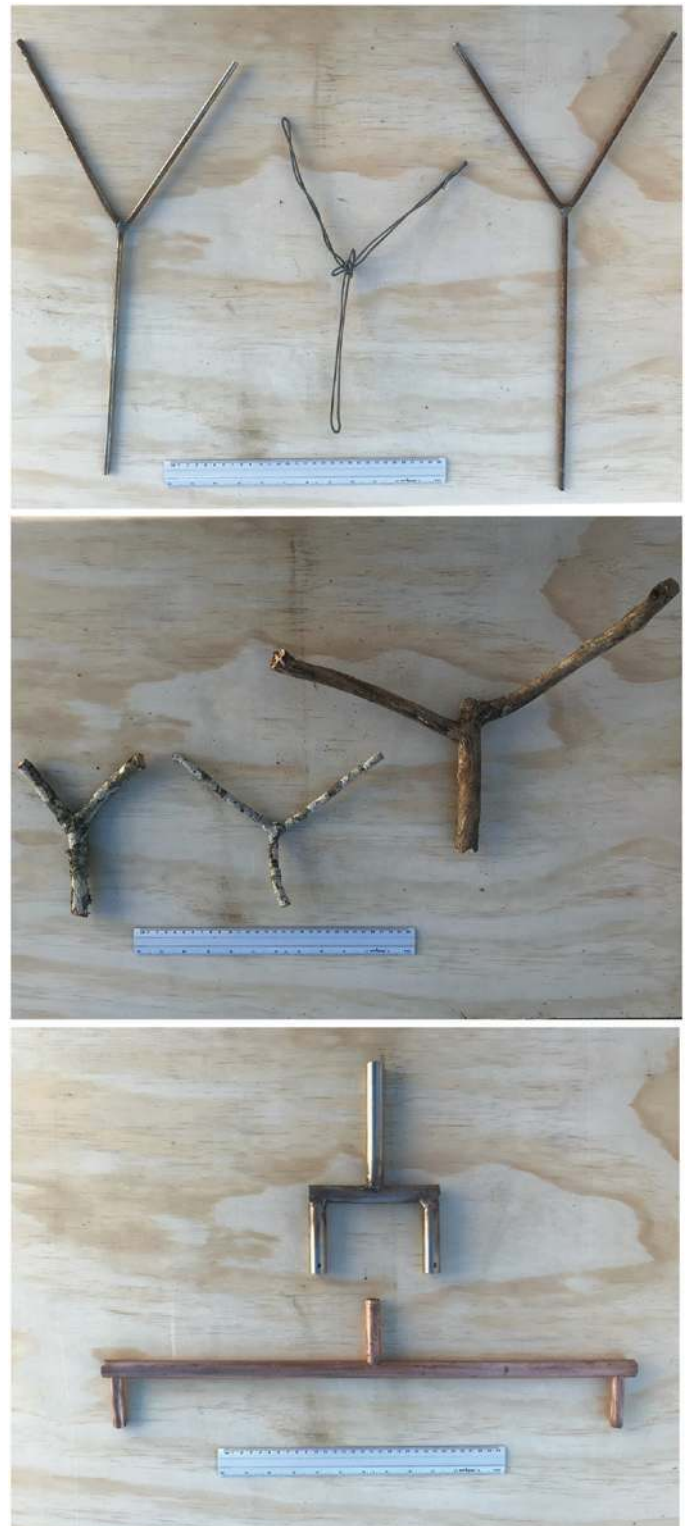
Figure 10. Divining rods constructed for field experiments. Top (left to right): no.1 steel, very high magnetic susceptibility ( \sim 130 SI), 165 gm mass; no.2 fencing wire, high magnetic susceptibility, 47 gm; no.3 stainless steel, non-magnetic, 176 gm; Middle (right to left) no.4 grey gum, 115 gm; no.5 yellow bloodwood 18 gm; no.6 jacaranda, 26 gm; Bottom orthogonal rods, no.7 stainless steel, non-magnetic, 287 gm; no.8 copper non-magnetic, 420 gm and 57 cm length. Scale 30 cm on each panel. Rods no.1, no.2 responsive to magnets, rods nos.1, 2, 3, 7, 8 highly conductive (ohmmeter test), rods nos.4, 5, 6 non-magnetic and resistive.
