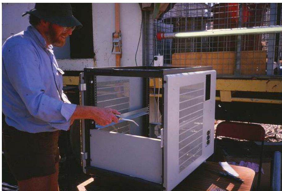
Mike Sexton "servicing" the HP1000 seismic processing computer with compressed air in camp during the 1988 BMR Canning Basin seismic survey. The computer had stopped working so Mike felt there was nothing to lose by stripping it down, removing all the cards and cleaning all the dust out before we sent it off to be repaired. However, when we re-assembled it and turned it on it didn't miss a beat for the rest of the survey!
