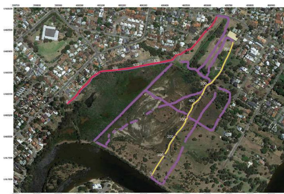
Figure 1. Overview of survey area in Perth, WA. All survey lines are shown in purple; the location of Line 4 is highlighted in red, the location of Line 5 is in yellow. Distances along Lines 4 and 5 are shown in white.
