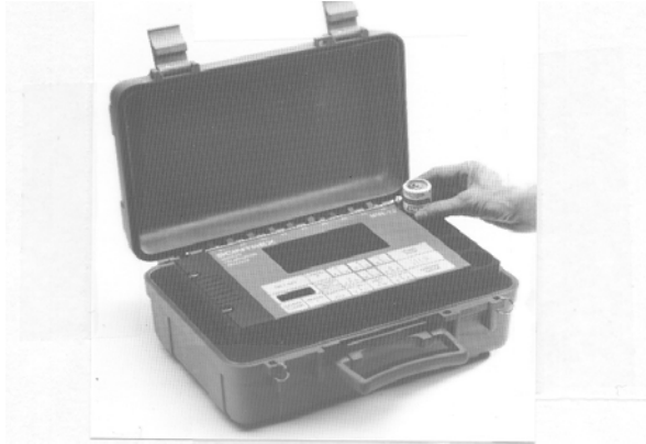
Figure 3: Installing The Batteries
