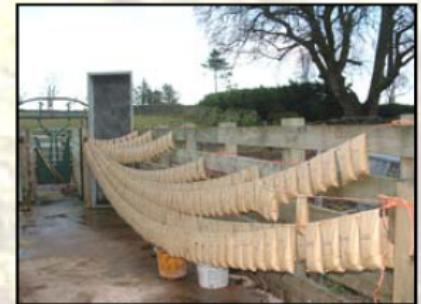
The samples are air dried until plastic in consistency, before being dispatched to Keyworth for freeze drying and sample preparation.
